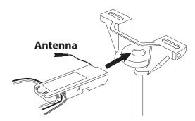
Gently insert the receiver into the Mounting Bracket with the flat part towards the top. Carefully push wires and wire connectors into the electric box leaving the antenna outside of the Mounting Bracket.
