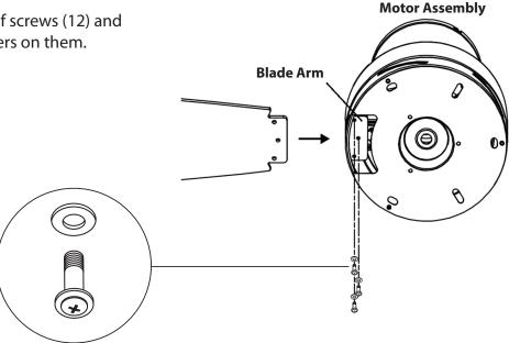
Insert the Blade through the rectangular slot in the Motor Assembly and align the holes in the Blade with the holes in the Blade arm.
