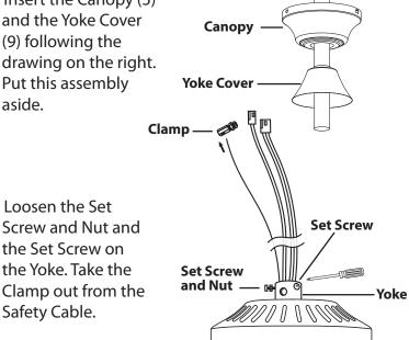
5. Insert the Down Rod into the Yoke making sure that the wires are not twisted and aligning the holes for the pin on the Down Rod with the holes in the motor Yoke. Insert Pin all the way through and put the Clip in place. Secure tightly the 2 Set Screws and Nut. Lower Yoke cover until it rests on
