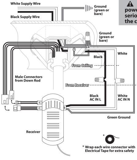
WARNING: Failure to disconnect power supply to the box may result in serious injury. Double check now that the circuit breakers to the box are off.
