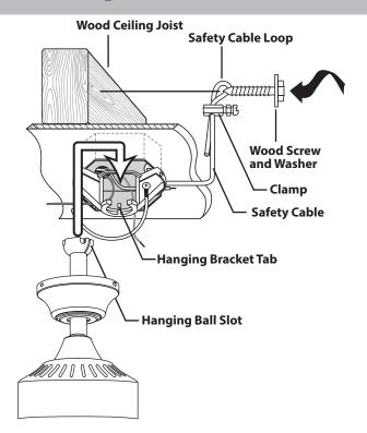
**WARNING: Failure to align** hanging ball slot with hanging bracket tab may result in serious personal injury or death.
