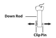
4. Thread the wires and safety cable that comes from the Motor Assembly through the Down Rod.
