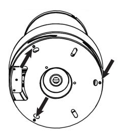
Connect the wires from the Lamp Base with the wires in the lower part of the Motor Assembly using the pre-installed electric connexions.
