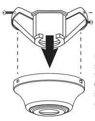
Partially loosen the screws in the slotted holes of the Canopy. Remove the other 2 screws from the Canopy/Bracket assembly. Twist and separate the Canopy from the Mounting Bracket. Save the screws.
